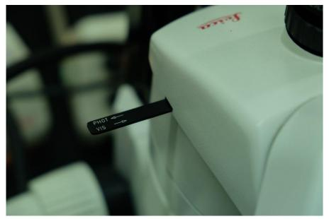
Pull out to take pictures. This redirects the light path for the right eyepiece to the microscope camera. In this mode, only the left eyepiece can be viewed through.
